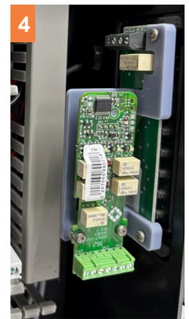
4 Tighten the two screws and press at the top of the driver to secure it and close the cable channel
