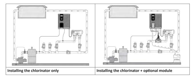
• The cell must always be the last element placed on the pool return pipe (see diagram).
