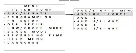
• 2 auxiliary devices can be controlled with the option of assigning one device as a lighting system:
