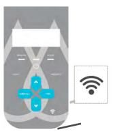
Once the connection with your home network is established, the appliance is connected to the Internet (WEB): the Wi-Fi LED is then lit steady.
