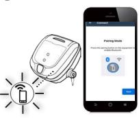
Press the ( button on the control box to enable Bluetooth™ and start the pairing process.
