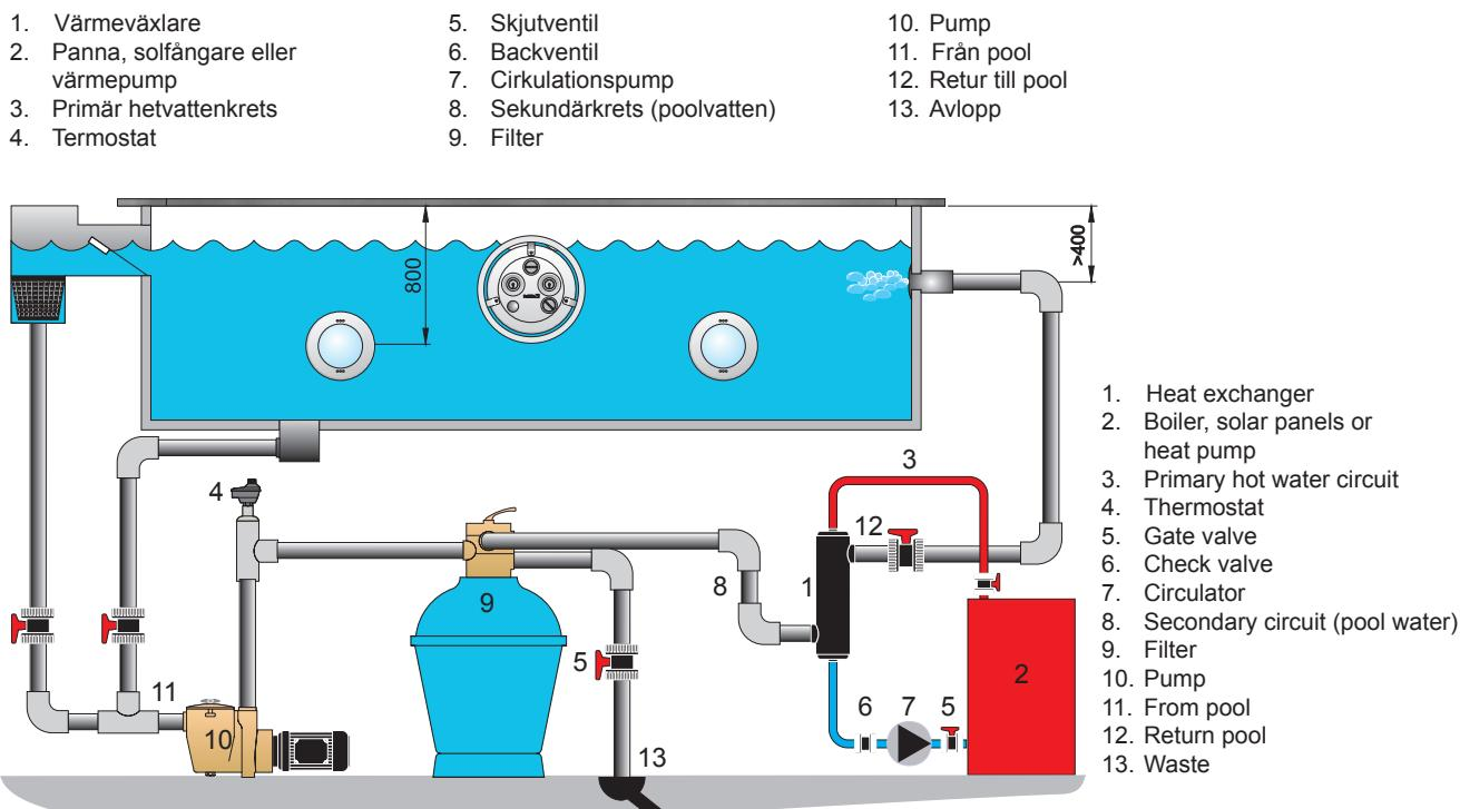
Install the heat exchanger according to the illustration.
