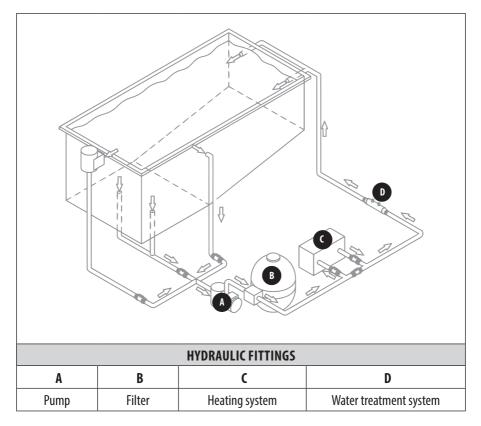
• Use as few elbow joints as possible. If there must be more than 10 elbow joints in the hydraulic circuit, the diameter of the piping must be increased.
